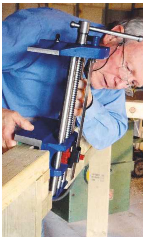
▲ Pic.4 Between the jointed cross rail is a free rail (here being hammered) and some roofing batten to make up the gap. Too many joints would have weakened the very area I was trying to strengthen. These pieces were then cut out for the vices and copiously screwed to each other
